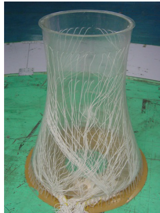
Fig.1b Model for internal pressure
