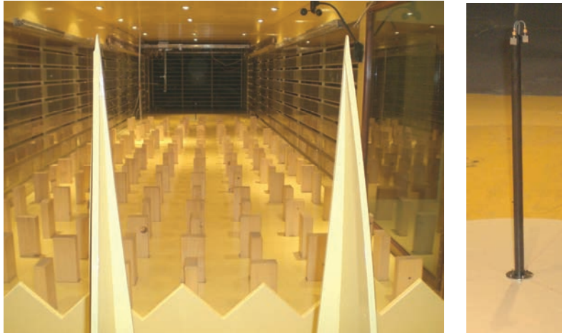
Figure 1. View of the wind tunnel with the model place on rotational table and one of the models.
