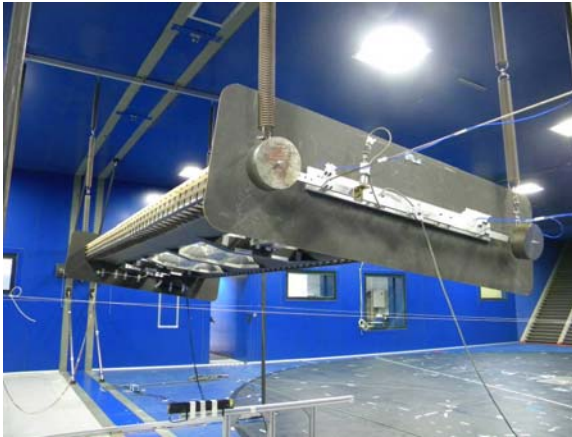
Figure 9. Free motion experimental set-up: Suspension system, tensioned steel stays and spring system.
